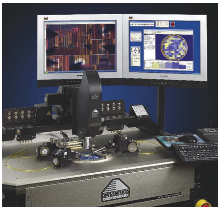
The eVue digital-imaging system for evaluation-wafer probing adds features that simplify setup, navigation, probing, and data correction.
