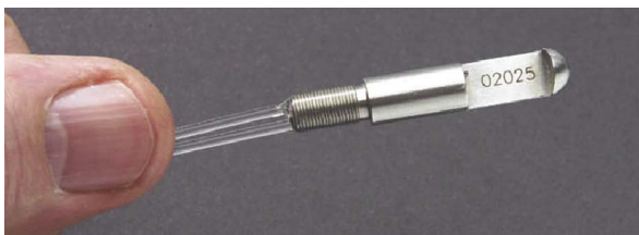
The Model 9732 ice-detecting transducer probe uses an infrared-laser diode and collocated photodiode to assess icing conditions, based on optical attenuation in the light path.
