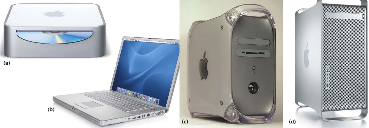
Figure 1 Apple's 1.25-MHz Mac Mini (a), 1.25-GHz G4 PowerBook (b), dual 800-MHz G4 Quicksilver Power Mac with GeeThree's Sweet Multiport installed (c), and dual 1.8-GHz G5 Power Mac (d) underwent intensive benchmark scrutiny during this hands-on project.
